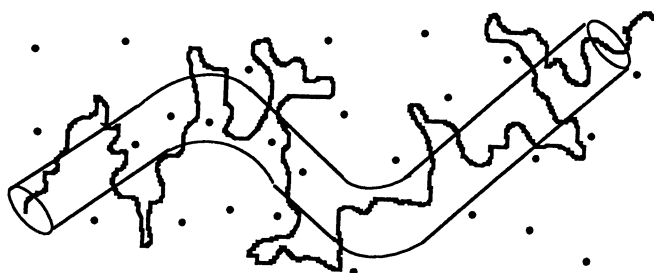
Figure 12 : Sketch of the tube model. The points illustrate the chains perpendicular to a reference chain represented by the solid line. The tube is due to entanglements, so that the polymer can only reptate along the tube [19, 29].
